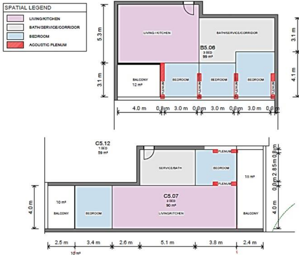
Figure 43: Plenums arranged in plan on the reference scheme.
